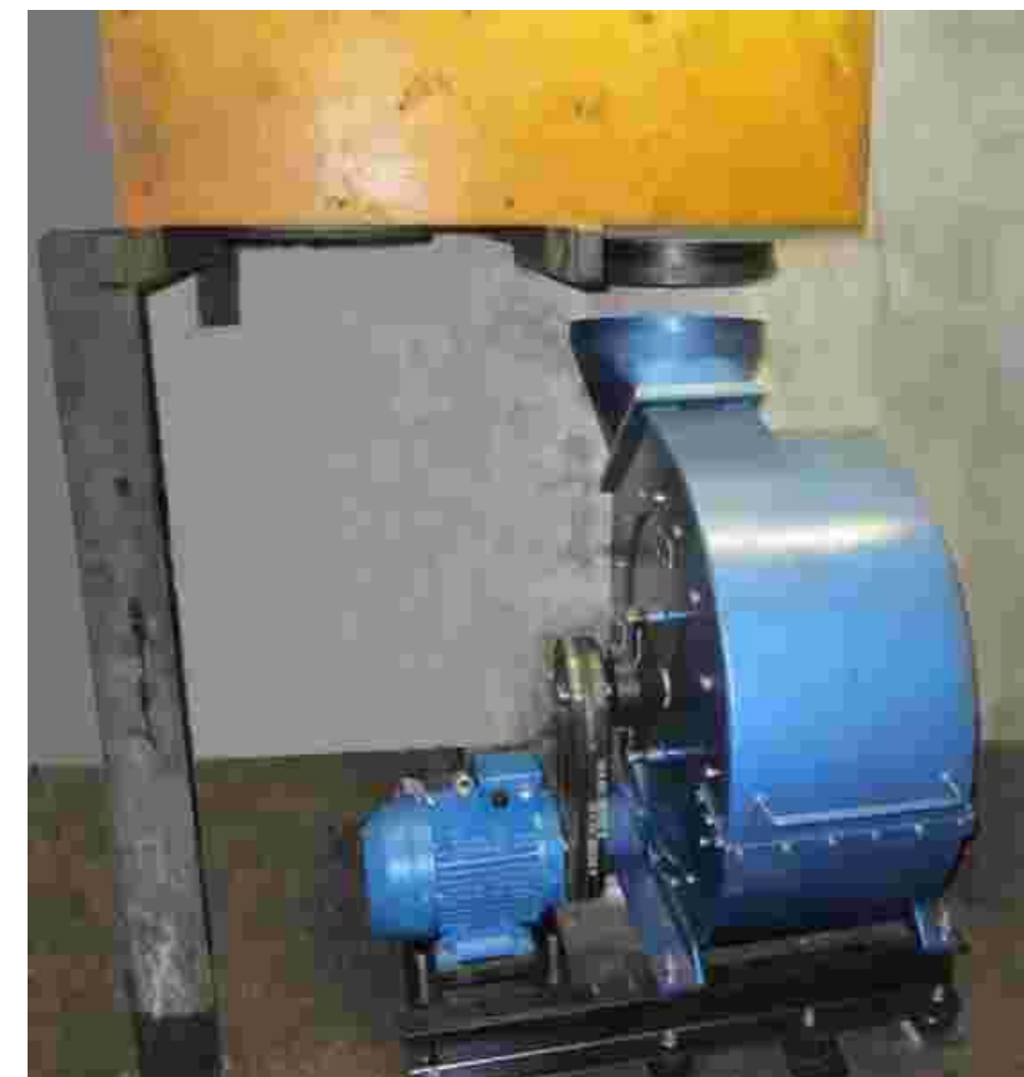
Organ fan - source of compressed air
